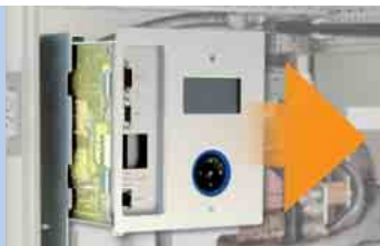
1. Control electronics are easy to remove.
